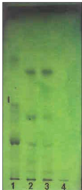
FIGURE 5: HPTLC finger print profile of C. angustifolia seeds and endosperm for identification of marker components with reference to Delcolex in UV254.
