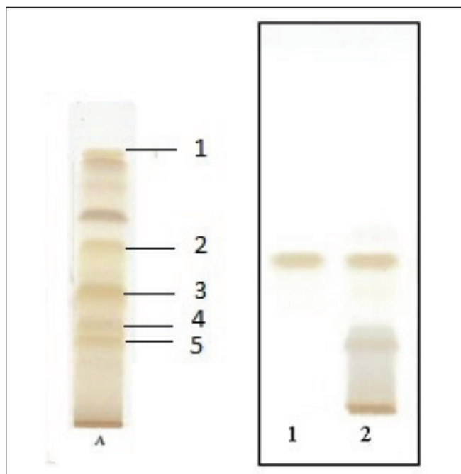
Figure 8: Typical ethyl acetate pattern of guava leaf. A: Ethyl acetate extract of guava leaf, 1: Quercetin, 2: Quercetin-3-O- \alpha -L-arabinofuranoside, 3: Quercetin-3-O- \beta -D-arabinopyranoside, 4: Quercetin-3-glucoside and 5: Quercetin-3-galactoside.
