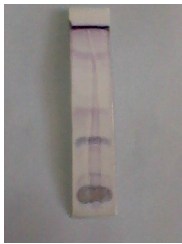
Figure 3: TLC of bark extract (n-Hexane: Chloroform) - 10 bands indicating the presence of alkaloids
