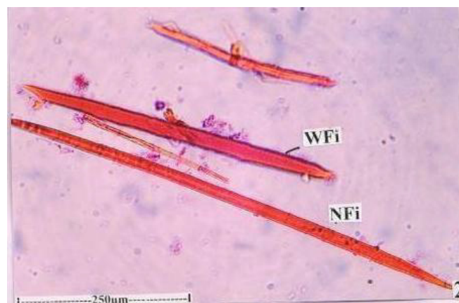
Figure 5.2 One narrow fiber and one wide fiber (NFi-narrow wide fiber, WFi-wide fiber).
