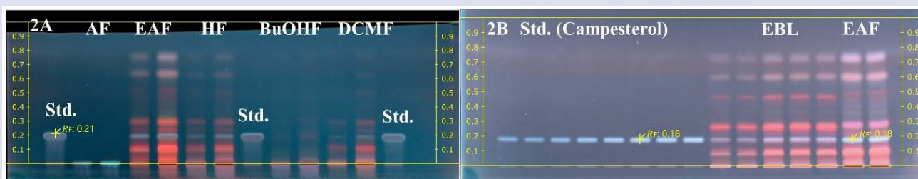
Figure 2: A) HPTLC fingerprinting analysis of all five fractions of EBL B) Quantification of campesterol in EBL and EAF.
